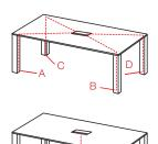
The distribution of electricity is entirely configurable; the exit for the cables can b placed inside any leg (A, B, C or D). Please specify the Customer Departmente which leg is to have the cables with reference to the view of the table in the diagram below.
